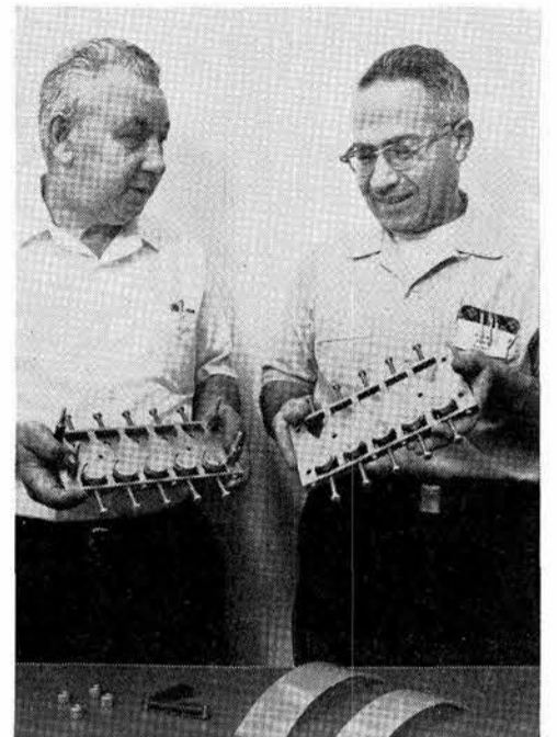
ED DLOUHY (2213), left, and Nick DeLollis (1133) display two halves of a new fixture used in preparing precise thicknesses of adhesive bonds for electrical characteristics testing. The halves are match-machined together to assure perfect alignment of positioning holes.
